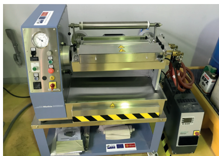
Lab-scale pad finishing system for fabrics
