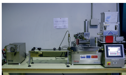
Lab-scale processing of biocomposites by twin-screw extrusion (0.5 kg/h)
