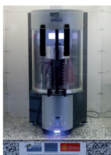
Tensiometer for the determination of surface properties of fibres
