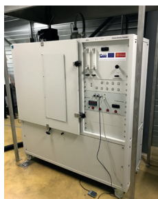
Analysis of smoke emitted during combustion
